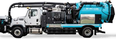
**Single Engine Combination Sewer Cleaning Truck**
