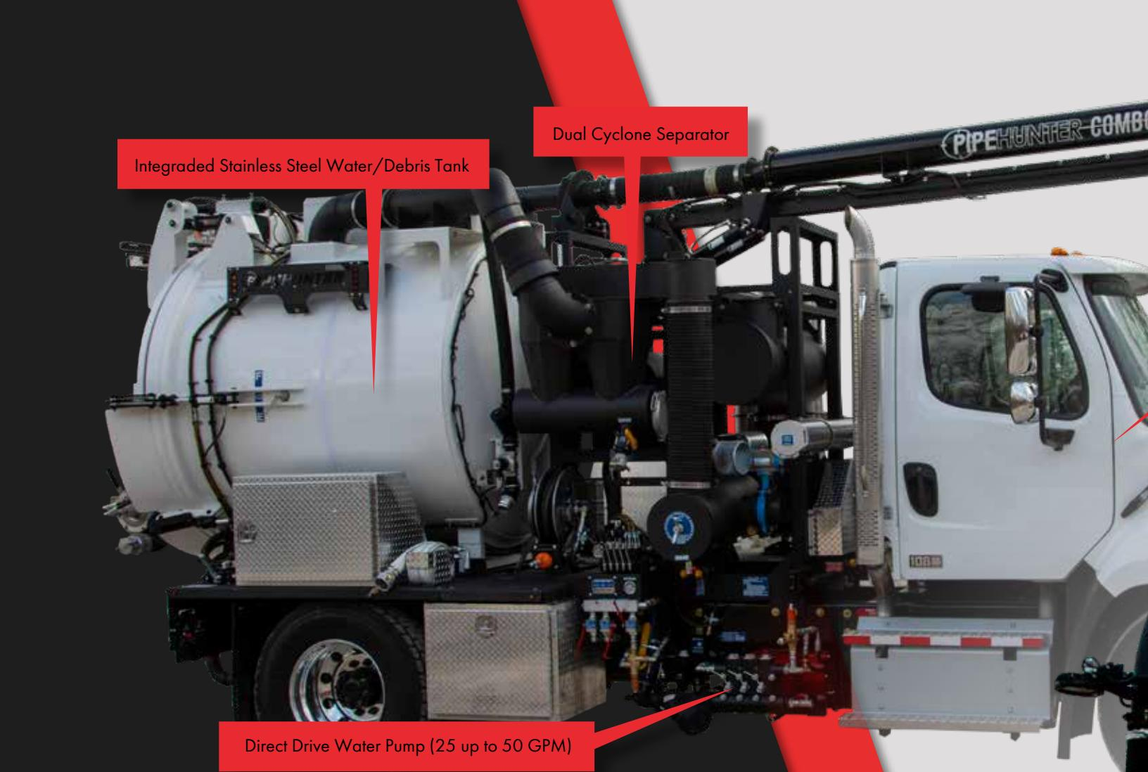
Integrated Stainless Steel Water/Debris Tank
