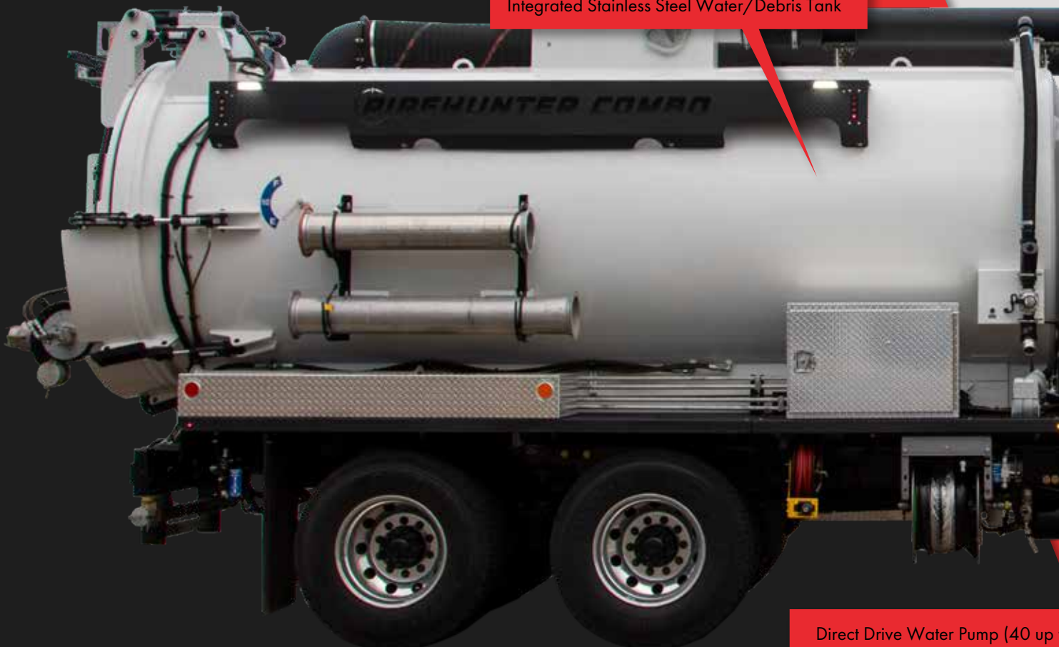
Integrated Stainless Steel Water/Debris Tank
