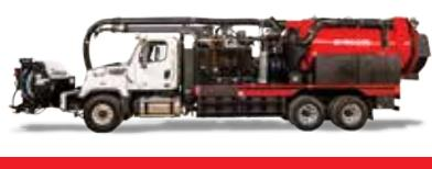
**Dual Engine Combination Sewer Cleaning Truck**
