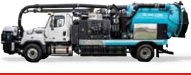
**Single Engine Combination Sewer Cleaning Truck**
