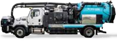
**Single Engine Combination Sewer Cleaning Truck**
