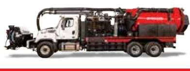
**Dual Engine Combination Sewer Cleaning Truck**
